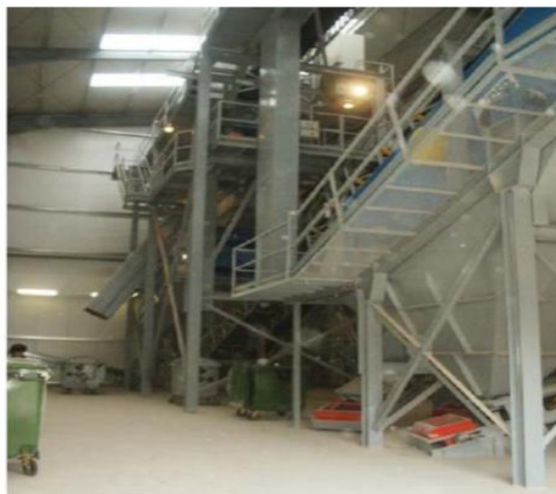
Figure 3. 20. Crushing, shredding and classifying machine line.
