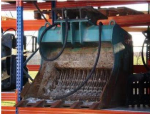
Figure 3. 27. VTN SB10 screening bucket.
